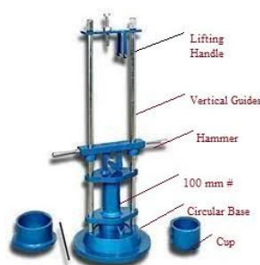
Fig. 4 The drop weight impact machine is shown in a systematic diagram
