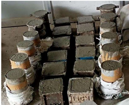
Fig 4. Casting of Specimens
