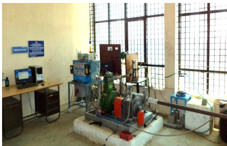
Fig. 1: Experimental setup of Diesel engine test rig
