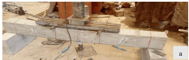
Fig. 14 : Flexural cracks failure for control (a)beam 1 and (b)beam 2
