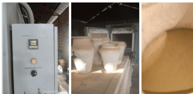
Fig. 1: Calcination of raw kaolin in furnace at the laboratory
