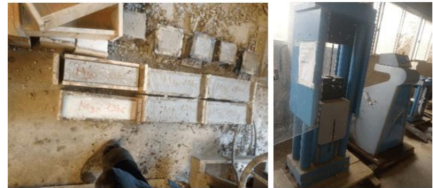
Fig. 3: (a) Prismatic specimens casted for experiment and (b) Steel rebars tensile testing
