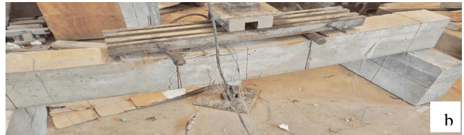
Fig. 14 : Flexural cracks failure for control (a)beam 1 and (b)beam 2
