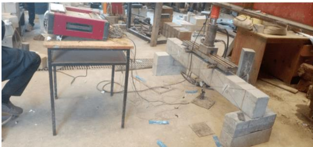
Fig. 8: Four-point bending experimental testing set up of RC beam
