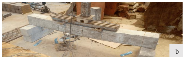
Fig. 15: Flexural cracks failure for beam 1&beam 2 with opt %CK
