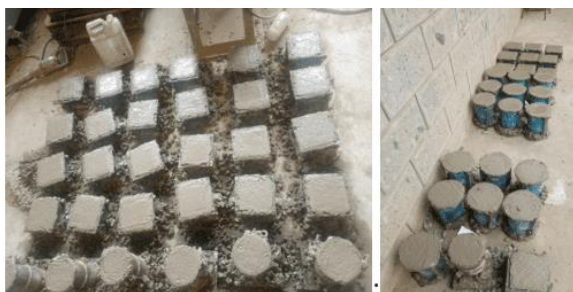
Fig. 2: Cubical and cylindrical specimens casted for experiment
