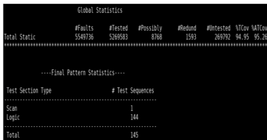
Figure 7: DC testmode coverage for RAM dominated block
