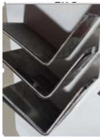
a)80 Degrees bending angle
