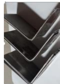
a)80 Degrees bending angle
