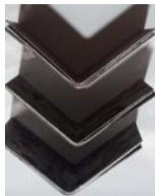
b)100 Degrees bending angle
