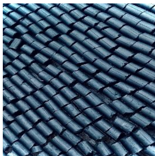
Figure 2. Briquette production process: (a) Briquette making machine and (b) samples of briquettes produced at 6.6 wt% binder ratio.
