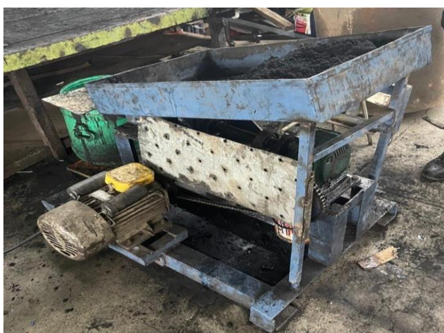
Figure 2. Briquette production process: (a) Briquette making machine and (b) samples of briquettes produced at 6.6 wt% binder ratio.
