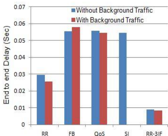
Fig.6. End-to-end delay with UDP traffic in the grid topology.
