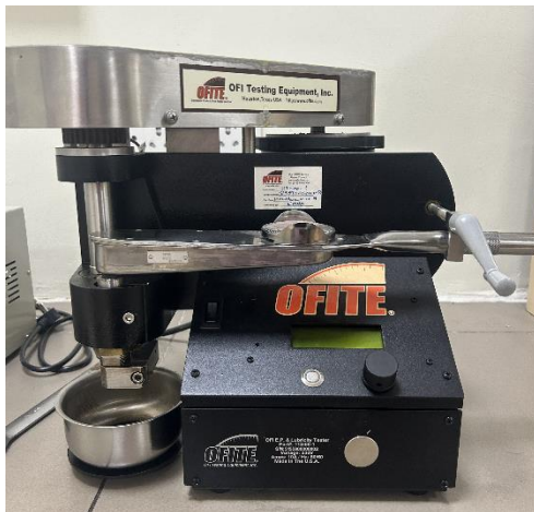
Figure 3. Lubricity tester ( OFI Testing Equipment, Inc.)
