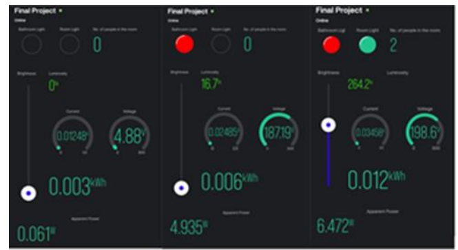
Fig. 11: Illustrates how power consumption rises as more appliances are used (left to right).
