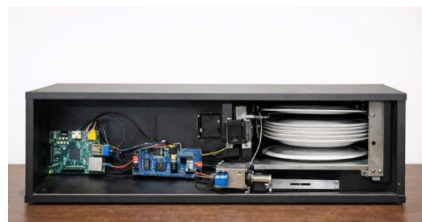
Fig. 4. Automated plate dispensing mechanism activated using relay-controlled solenoid lock.
