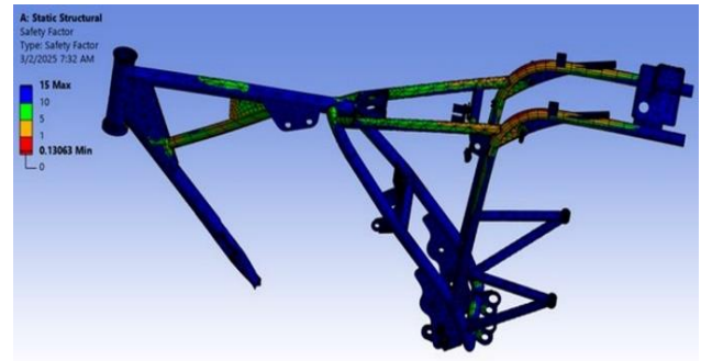
Figure 8. Analysis of safety factor (Life) of the motorcycle frame under load conditions
