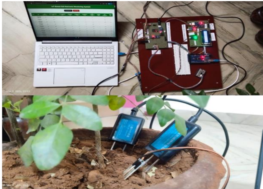
Figure 5. Hardware Implementation of IoT-Based Soil Nutrients Monitoring System – Sensors all inserted into the soil, and reading of nutrients displayed
