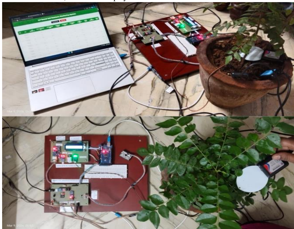
Figure 6. Hardware Implementation of IoT-Based Soil Nutrients Monitoring system, also checking the pollution, leaf wet, and temperature.
