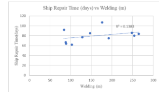
Fig 5. Welding vs SRT
